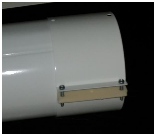
Fig. 6 Extension pipe for a 'connection' joint'
