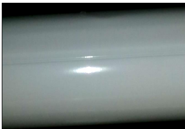
Fig. 1- Laser welded longitudinal seam
