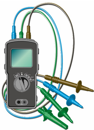
Figure 2 – An example of an Earth Fault Loop Impedance Tester
