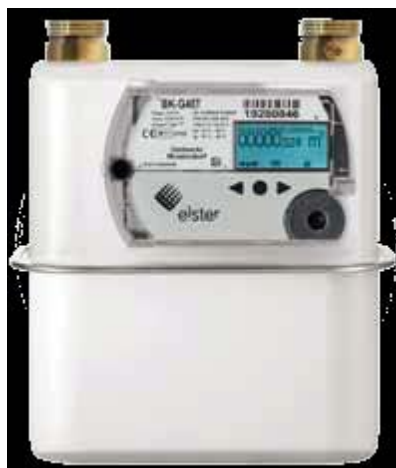
Figure 1 shows a typical Elster diaphragm smart meter. The meter uses a traditional base Kromschroder G4 meter with a smart module in place of the mechanical index.
