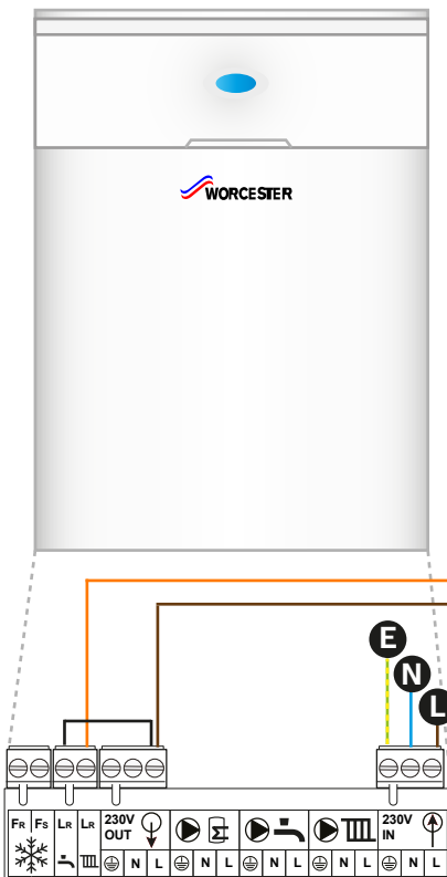
Wiring Terminals Inside Boiler
